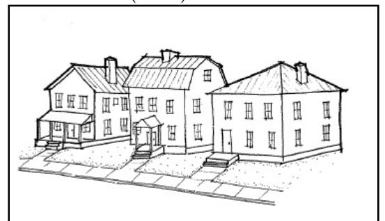
New construction with incompatible setback and foundation height.
