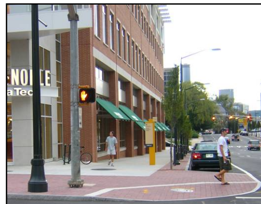
Use of awnings and windows, arranged like storefronts, helps to make a large new building compatible with the scale and design of historic buildings.
