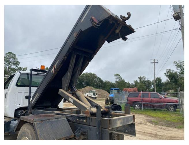
Hoist capable of transporting and dumping 11 Ton swaycar trailer loads.
