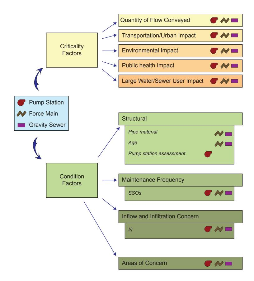
Figure 2-1: Condition and Criticality Factors and Their Applicability to Wastewater Collection System Assets
