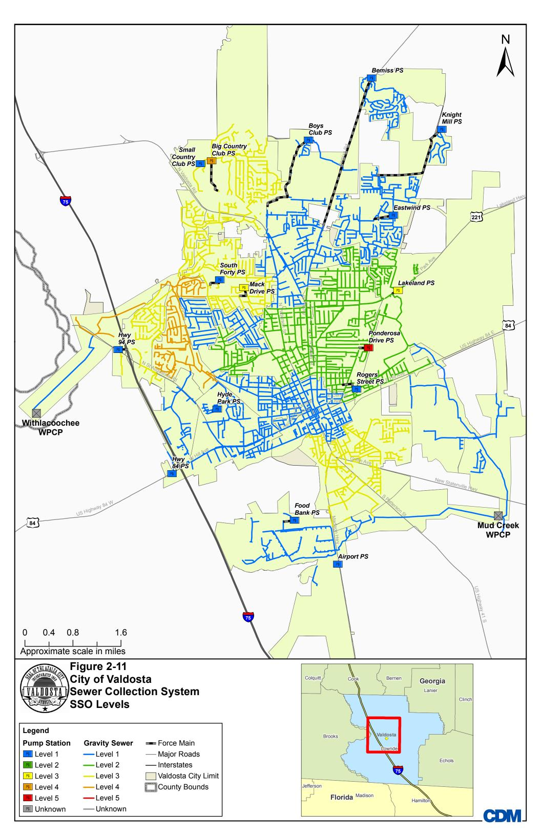
The model predicted peak wastewater flow recorded during the storm event was compared with the average dry-weather flow (ADWF) recorded at each temporary flow monitor. The highest levels were assigned to gravity sewers within the sewersheds upstream of the monitors that had the highest peaking factors. All gravity pipes within the sewershed were assigned the same level. Pump stations with high I/I were identified based on peak flows within the sewershed.
